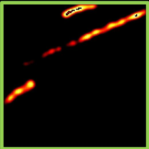
Image credit: machine learning predictions for displaced molten material (spatter) in metal alloy laser powder bed fusion (LPBF). This semi-supervised learning technique allows pixel-by-pixel classification with high-speed thermal camera imagery. Sean Tronsen, Colt Montgomery and Nathan DeBardeleben, Los Alamos National Laboratory.
